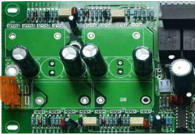
UPS Power Board UPS电源板
